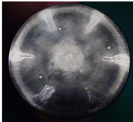
Figure 4. Pitted Surface on Lifter Face, Abnormal Condition
