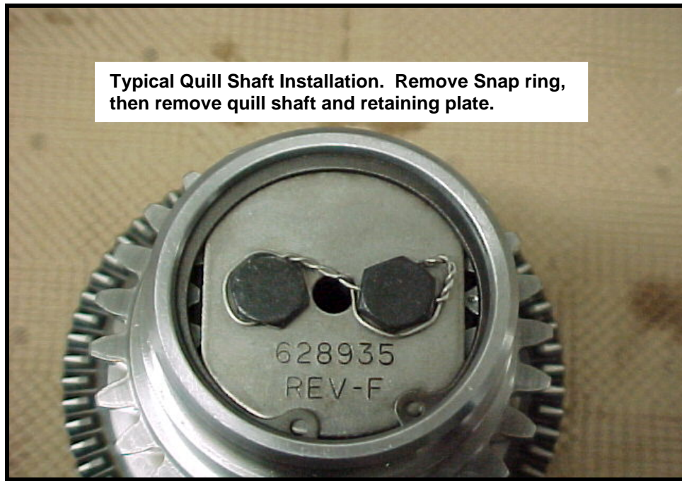
FIGURE 3. QUILL SHAFT INSTALLATION
