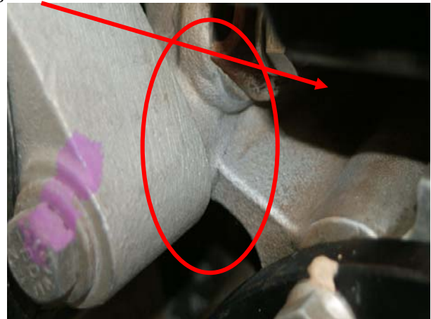
FIGURE 3 Compressor bracket attachment bolt boss crack indication
