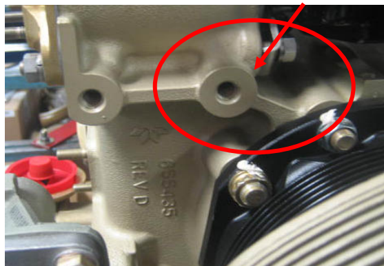
FIGURE 5 Thinner Rib (Approximate thickness 3/8")
