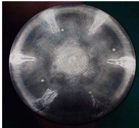
Figure 4. Pitted Surface on Lifter Face, Abnormal Condition
