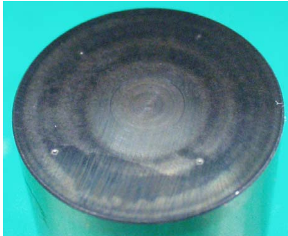
Figure 6. Normal Lifter Face Wear Patterns
