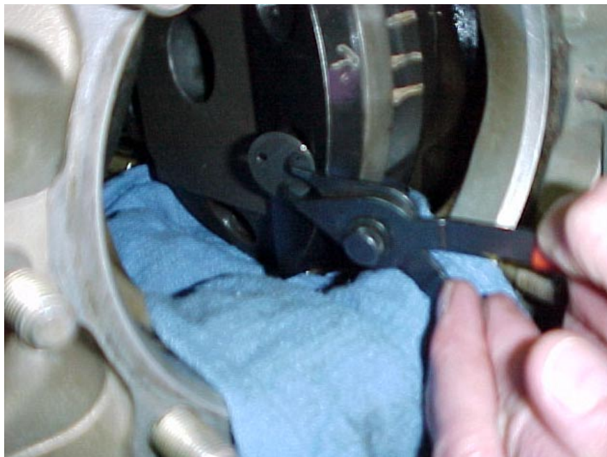
FIGURE 2. REMOVING COUNTERWEIGHT RETAINING PLATES
