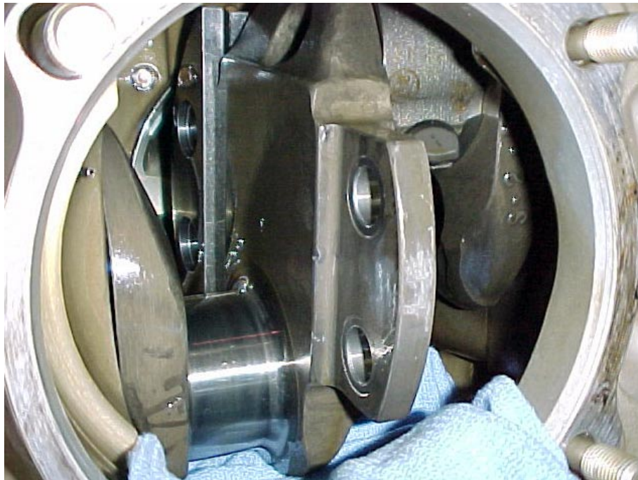
FIGURE 7. CRANKSHAFT COUNTERWEIGHT BLADE
